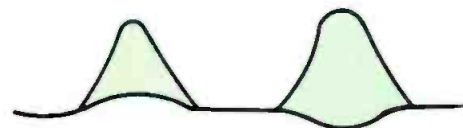
Figure 3. Vertical bowing of the composite baseline indicates amplitude errors. A waveform such as this indicates low B-Y and high R-Y amplitudes.
